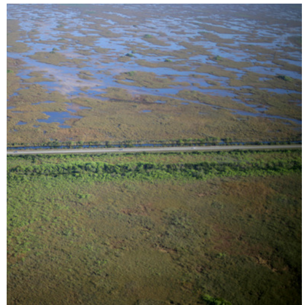
The Tamiami Trail highway blocks the natural flow of water through the system. Elevating sections of the highway would allow the water to flow more naturally. Photo: Lori Oberhofer, Everglades National Park
